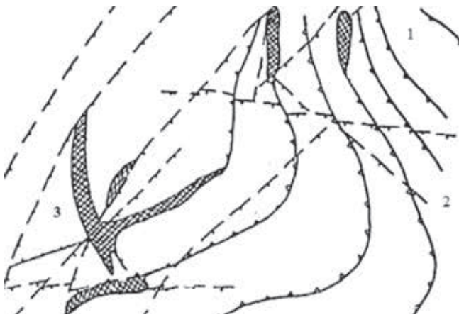
Fig.1. Structure of the Ishimskoye deposit (Kazakhstan): 1– tectonic disturbances; 2–layered deposits; 3– ore bodies
