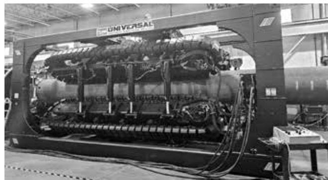
Picture 9. Pipe feeder of Universal HDD at factory tests in the shop at Lake Zurich, IL
