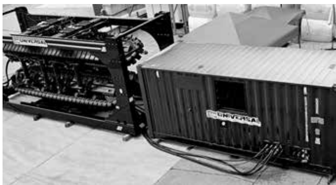
Picture 4. Pipe feeding device built by Universal HDD in 2024
