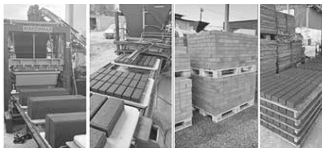
Fig. 4. Mobile workshop for the production of ash and slag products of Politech Construction LLP and finished products
