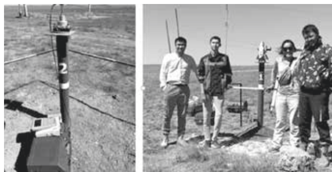
Fig. 8. Monitoring by GPS receivers and electronic tacheometers Basic (reference) point installed at permanent forced centering points
